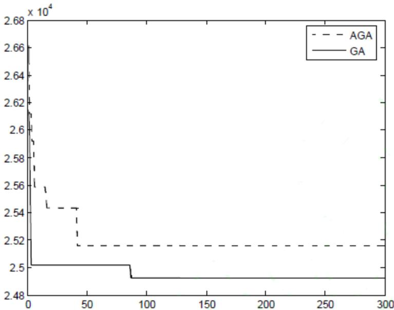
Fig. 4. Convergence graph of adaptive genetic algorithm for scheme 1
